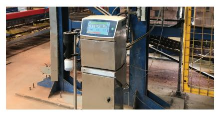
A UK based brick and concrete producer uses PrinterNet to remotely access their Linx 8900 printer located outside a safe area of their factory. The production line stops if the light beams in front of the printer are broken so being able to create and amend messages remotely is a perfect solution.
