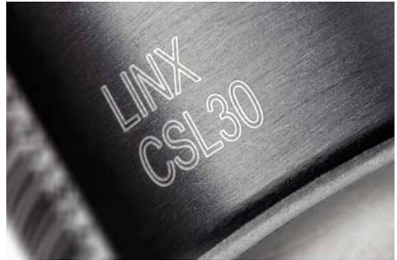
Laser coding of coated aerosols
