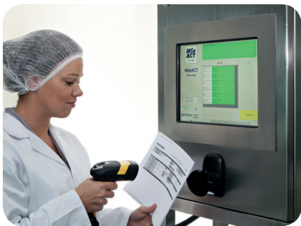
Hand scanner can barcode scan a production plan pack list to “start the job”.
